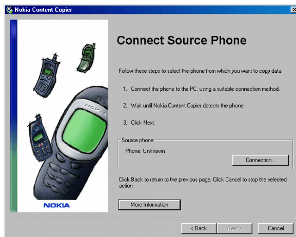
Figure 1. Connecting source phone and selecting the connection type for it.
